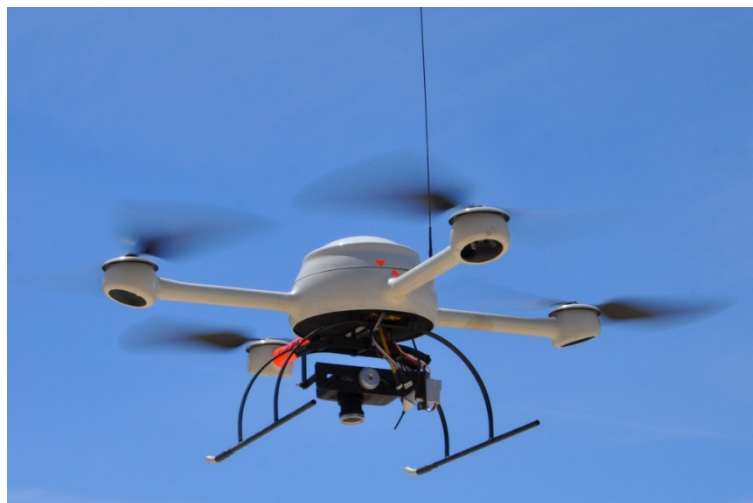
Figure 1. The commercial “ready-to-use” Microdrones MD 4-200. Payload includes IMU, GPS receiver, downward pointing CIR-modified digital Canon IXUS 100 camera, radio downlink and microprocessor controlled flight control units.
